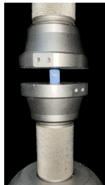
Figure 5: Measurement of gel strength and permanent deformation using universal testing Machine
