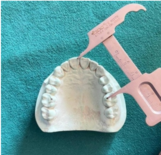
Figure 6: Dimensional accuracy measurement using vernier calliper
